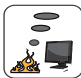
Low Corrosivity IEC60754-2 EN50267-2-2/3 NF C 32-074
