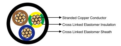
**Conductor:** Stranded bare copper.
