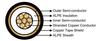
**Conductor:** Stranded bare or tinned copper conductor.
