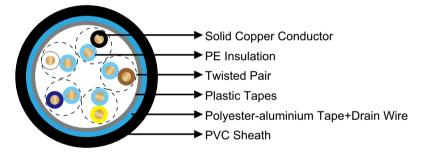
Conductor: Solid bare copper.
