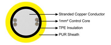
Conductor: Stranded copper conductor, Class 6 to VDE 0295/IEC 60228.
