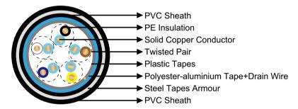
Conductor: Solid bare copper.
