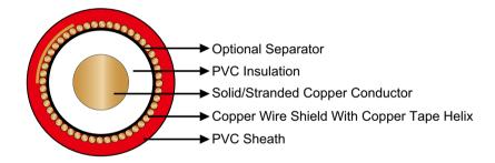
**Conductor:** Solid or stranded bare copper conductor.
