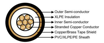
**Conductor:** Stranded bare or tinned copper.
