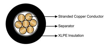
**Conductor:** Stranded bare copper to ASTM B3 and ASTM B8.
