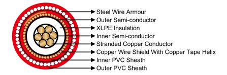
**Conductor:** Stranded bare copper conductor.
