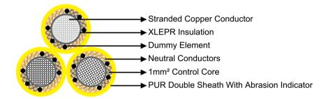
Conductor: Stranded copper conductor, Class 6 to VDE 0295/IEC 60228.
