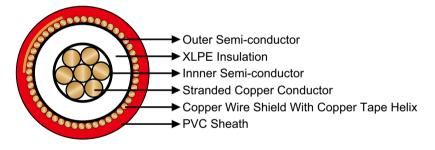
Conductor: Stranded bare copper conductor.
