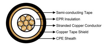
**Conductor:** Stranded tinned copper conductor.
