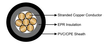
Conductor: Stranded bare or tinned copper conductor.
